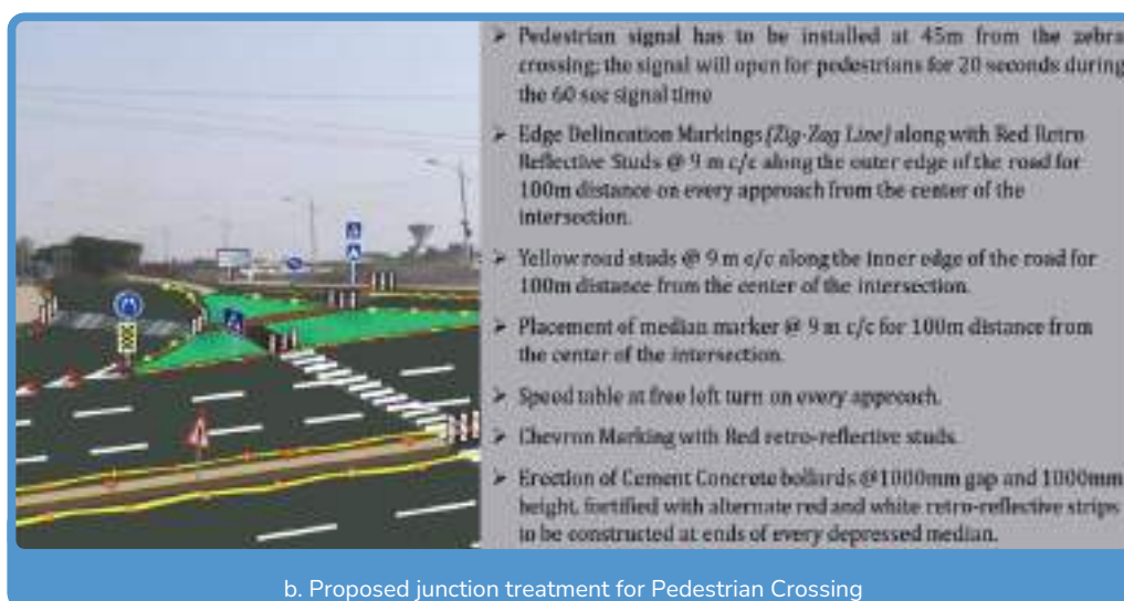
Figure 4.94 Pictorial Illustration of Few of Geometric Design Plans proposed at Chikli Square for Option 2
