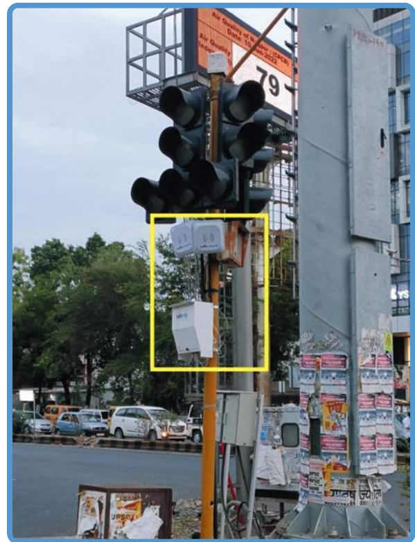
Figure 8.1 RFID scanners installed on Traffic Signal.
