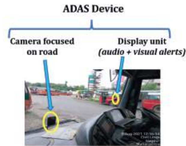
Figure 2.2 ADAS-enabled bus; The main components of an ADAS device include a camera unit focused on the road and a display unit.
