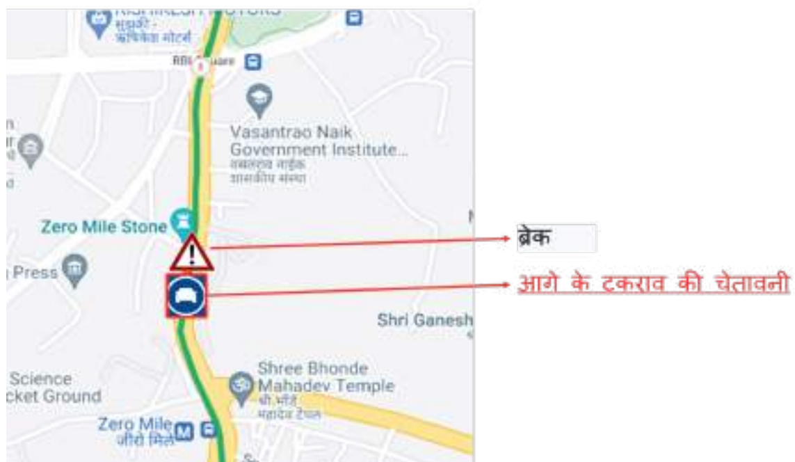
Figure 2.5 Driver applying hard brake, alerted by a FCW. Offline analysis based on cloud portal data
