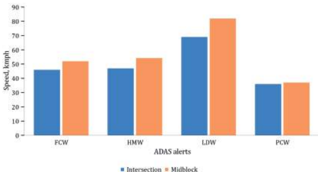
Figure 3.11 Comparison of the speed of ADAS alerts on Intersections and Midblocks
