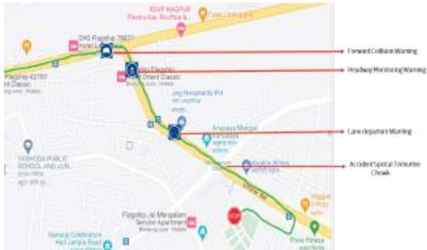
Figure 2.20 Illustration of ADAS alerts recorded prior to a crash
