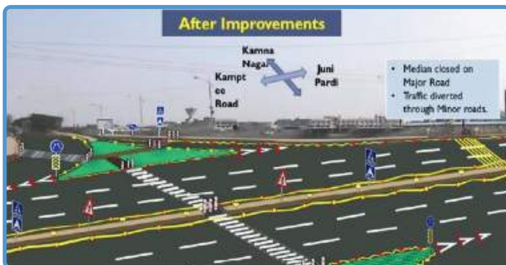
Figure 4.102 Typical Illustration of Chikli Square Option 2 having Junction Closure on the Major Approach.
