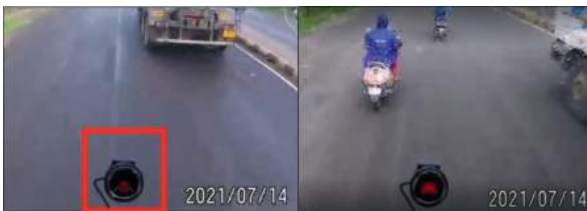
Figure 2.3 ADAS unit alerts driver with unsafe distance warning for VRUs; Pedestrians and Vehicles, including 2- wheelers are detected
